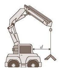
The distance, d, is measured to the front of the cab.
