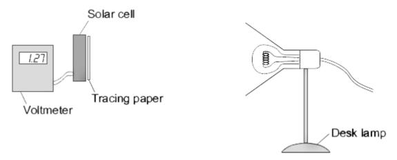
The student put the desk lamp a fixed distance from the solar cell. To represent the effect of a dirty surface, the student covered the surface of the solar cell with pieces of tracing paper. Each time the student added a piece of paper, she measured the output voltage of the solar cell.
