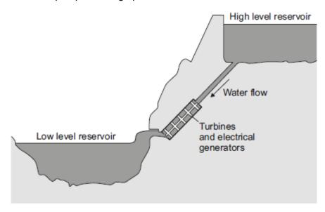
When electricity is needed, the water in the high level reservoir is allowed to flow to the low level reservoir. The flowing water generates electricity.
