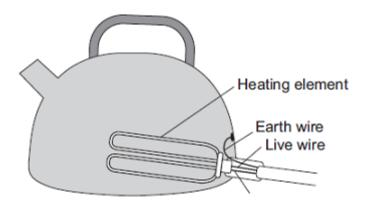
If a fault makes the metal case live, the earth wire and the fuse inside the plug protect anyone using the kettle from an electric shock.
