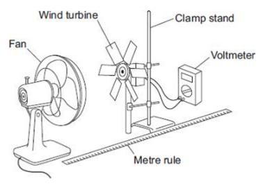
The fan was used to turn the wind turbine.
