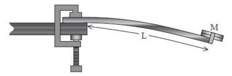
When M is displaced, the period of oscillation T of the cantilever is related to L and the Young modulus E of the material of the metre rule by the following equation:
