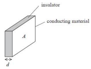
The capacitor has a capacitance 0.1 µF and is charged to a p.d. of 100 V by connecting it to an electrical supply.
