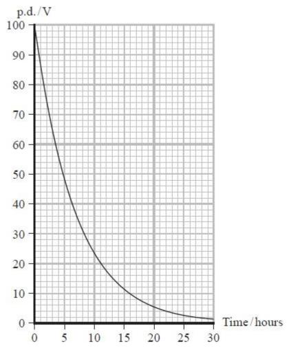
The insulator is a type of plastic and should have a resistivity greater than  $10^{14}~\Omega$  m. Deduce whether the plastic used in this capacitor has a resistivity greater than this value.
