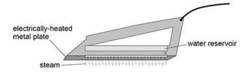
Water from a reservoir drips onto an electrically-heated metal plate. The water boils and steam
