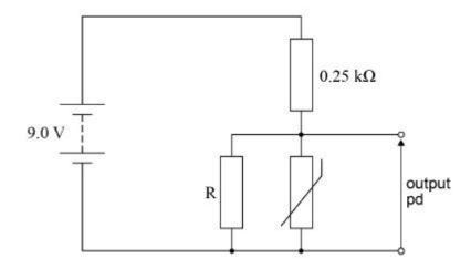
The supply has negligible internal resistance and the thermistor has a resistance of 750  $\Omega$  at room temperature. The student wants the output potential difference (pd) at room temperature to be 5.0 V
