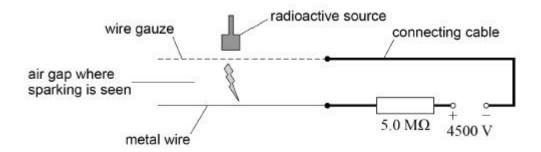
Sparks are produced when alpha particles produce ionisation in the air gap.
